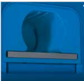
Sound isolation using Elodur® elastomer support for superior impact sound insulation.
