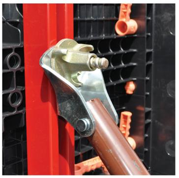
The shoring is performed using a steel bracket to connect the push-pull props to the formwork. The brackets are available in various sizes to suit any commercially available prop.
